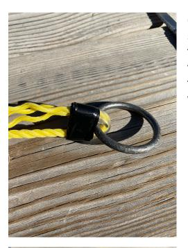
6.Slide the cord and tubing through a steel Schweizer or Tost link (larger of the two rings on the Tost) and fold the loop together around the ring. Tape the tubing to hold it in place while you splice the cord.
