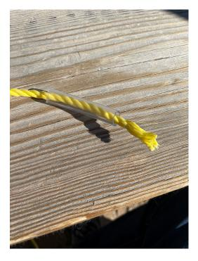
3.Cut a piece of 5/16 ID tubing about 2 inches long and place it over the piece of polypro cord.
