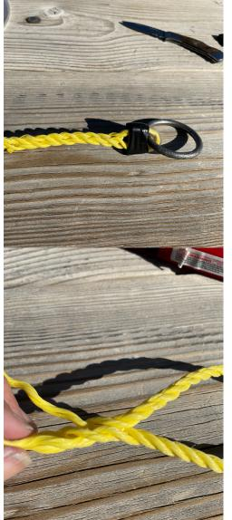
7. Make an eye splice on the cord as close to the tubing as you can, following the example shown in the video at:
