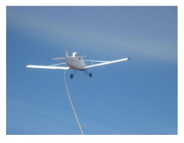
Return to Bottom Center: Control your pitch and elevation references while sliding back to bottom center. Rudder work is needed to effectively stop the slide to center without overshooting. Note the tail wheel is centered between the main wheels, just slightly above the wing reference line and the horizontal tail is positioned just slightly above the wing struts.
