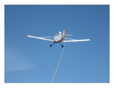
Top Left Corner: This is the top left corner of the box. Note that the as the glider ascends the tail wheel descends and maintains the same side to side reference with the right main tire. Also note that the Pawnee is back on the horizon. Left rudder and some slight bank away may be required to maintain this reference. The task is to climb the left side of the box from the lower left to the upper left without drifting left or right.
