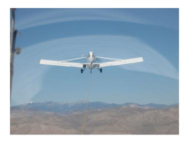
Transition to Low Tow: Transition straight down through the wake until the wake turbulence is no longer felt. For the Pawnee, the reference shows the tail wheel still centered between the main tires but is now up just above the wing line. Note the position of the horizontal tail just above where the Pawnee wing struts attach to the fuselage.
