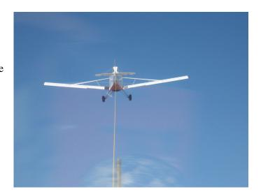
Finish the maneuver by transitioning smoothly back up through the wake. Continue the climb and stop with the Pawnee back on the horizon in the normal tow position. Be careful not to overshoot and get too high, but don't stop too low either.
