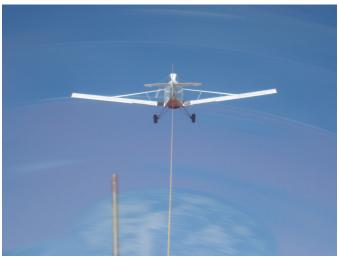
Bottom Left Corner: Slide left. Left rudder is required to slide to the lower left corner while maintaining the same elevation reference. Some slight bank in the direction of the skid may be needed to assist. Note that the tail wheel has maintained the same reference just above the wing and is now over the right main wheel. Also the horizontal tail is in line with a white trim panel on the pilot's left window.
