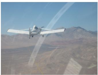
Bottom Right Corner: This can be the hardest transition. Top-right to bottom-right corner. The tail wheel moves up above the wing with the same "left / right" reference to the main wheel that you had at the previous "top right corner" position. A little bank and rudder coordination is required to maintain the left-right reference while in the descent. Note also that the Pawnee horizontal tail is again just above the wing strut and aligned with the white stripe on the pilot's side window.
