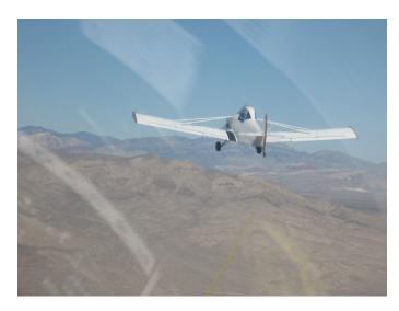
Top Right Corner: A level slide across the top of the box. Rudder work and stopping the slide with the tail wheel now positioned over the Pawnee left main tire. Don't slide too far or stop too early, it's hard to push out to the corner. Don't climb or descend, this is a level maneuver. A lot of rudder and a little bank may be needed to maintain this position.
